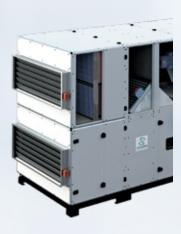
There are three different damper sections in the devices; suction cell with single damper, mixing cell with two (double) dampers and mixing cell with three dampers and they can be used according to the principles of the application. All dampers in the mixing cell dampers have been selected according to the velocities that will emerge when all the air is passed over them. Optionally, pre-filtering can be applied to damper cells.
