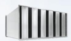
Control dampers with aluminium profile bodies and aluminium aerodynamic blades are used in the AIR HANDLING UNITS. The plastic gear mechanisms of the opposing blades are hidden between the aluminium edge profiles.
